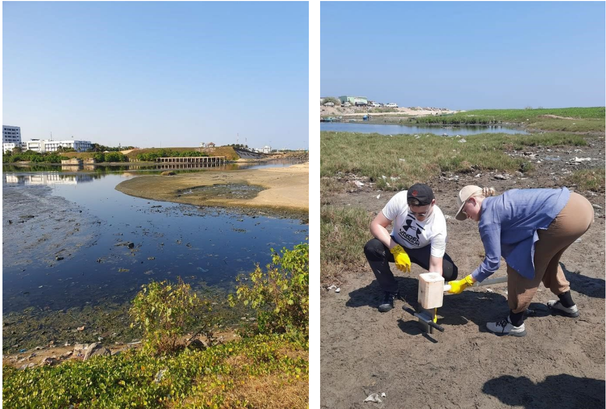
Figure 1: Sampling point Cooum river mouth (left); Sampling sediment samples with the Geoslicer (right)
