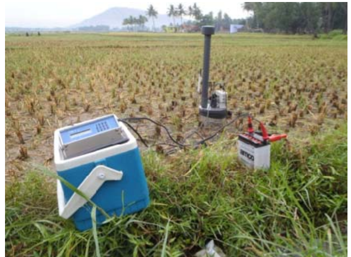
In-situ soil respiration measurement using a PP-Systems respiration chamber together with field infrared gas analyser
